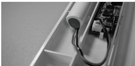
Figure 7. EXIDUS battery connection
